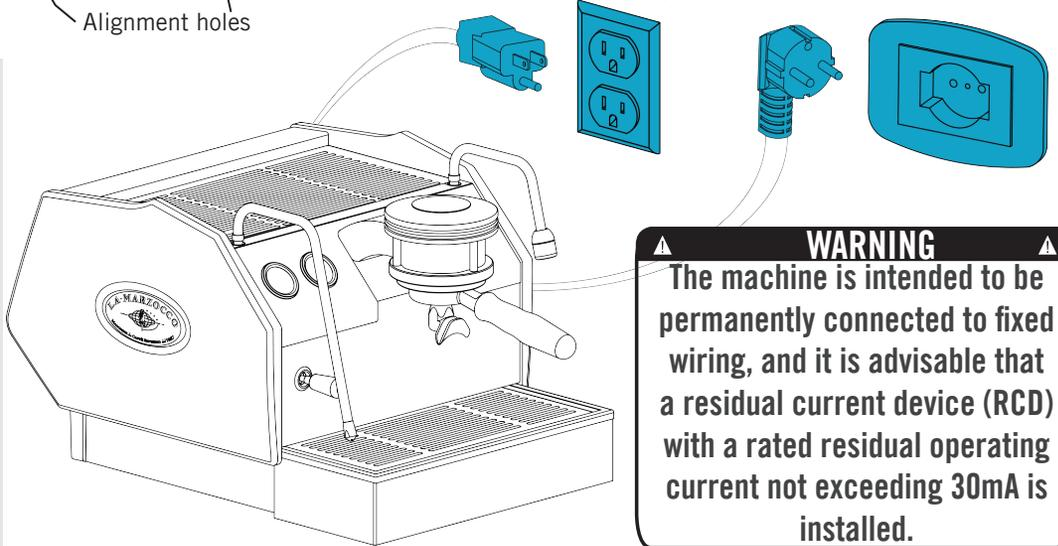
**4** Connect the power cord to power supply capable of supplying: 230 VAC and 10 amps (for the 230 V version) or 120VAC and 15 Amps (for the 110 V version).
