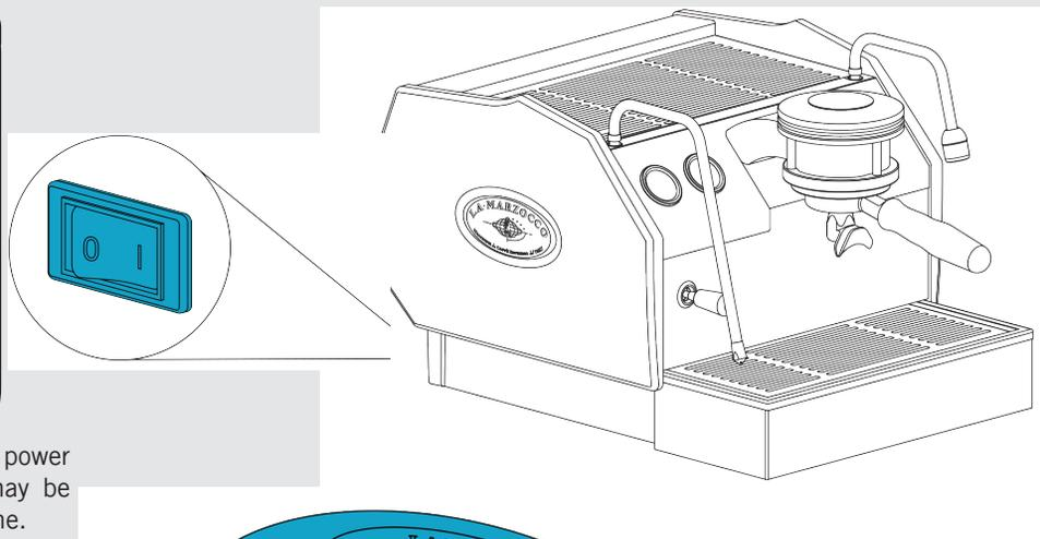
**5** Turn on power by pressing the main power switch. The main power switch may be found on the left rear of the machine.
