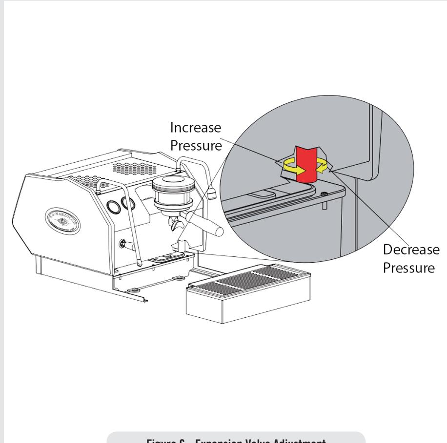
Figure 6 - Expansion Valve Adjustment
