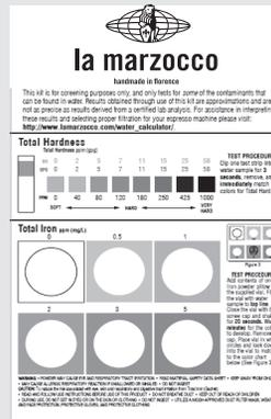
In order to enable you to check if your water supply is within the suggested ranges, La Marzocco machines will be equipped with a quick water test kit (see image below) including 6 test-strips and instruction cards.
