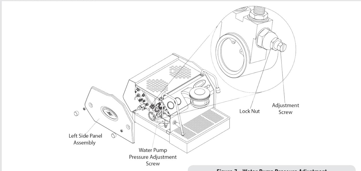
Figure 7 - Water Pump Pressure Adjustment
