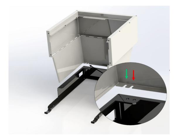
In order to add clearance around the pump motor, the screw position has been moved. Both the frame and the panel have 2 positions for holding the screw. This is in order to guarantee the interchangeability with previous frames or panels.
