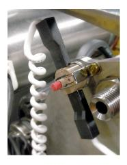
Please pay attention when connecting and disconnecting the thermostat, as the new cover, even though more resistant to temperature, is more fragile and could crack if not handled correctly.
