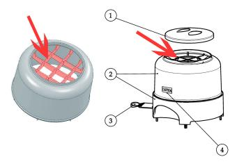
The shape of the inlet hole has been modified to facilitate easier loading of coffee. The new grid (shown on left) is positioned a step below the rim unlike the previous design (shown on right) and includes the same geometry as that of the Vulcano Swift hopper.
