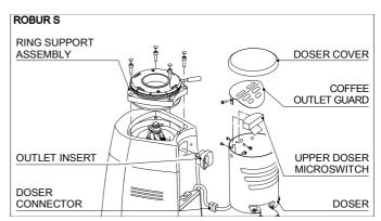
Remove the hopper and, after having unscrewed the relevant screws, remove the ring support assembly.
