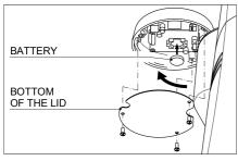
Here is how to proceed to replace the buffer battery:
