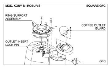
Remove the hopper and, after having unscrewed the relevant screws, remove the ring support assembly. Rotate counterclockwise the display cover, and remove the coffee outlet guard. For grinder with round GFC (Grind Flow Control), rotate a few degrees counterclokwiswe the GFC until it can be removed. For grinder with square GFC, remove the locking pin and out the GFC.
