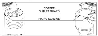
The coffee outlet guard must always be fixed to the doser (Grinder-Dosers), or to the funnel (Electronic Grinder-Dosers), using the relevant screws, which must never be removed by the user. The removal of the coffee outlet guard can be done by skilled technical personnel only after disconnecting the appliance from the power supply by unplugging. Before reconnecting the
